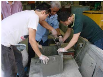
Placing & vibrating mortar
